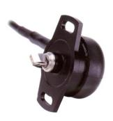
The output of a rotary potentiometer is a voltage which changes in direct proportion to the shaft angle. A constant voltage is required across the supply and ground wires of the sensor. No internal end stops are fitted, so continuous rotation is possible. Various lengths of electrically active track are available, up to a maximum of 340°. All units are sealed to keep out dirt and dust but some models can be fully sealed against the ingress of fluids.
